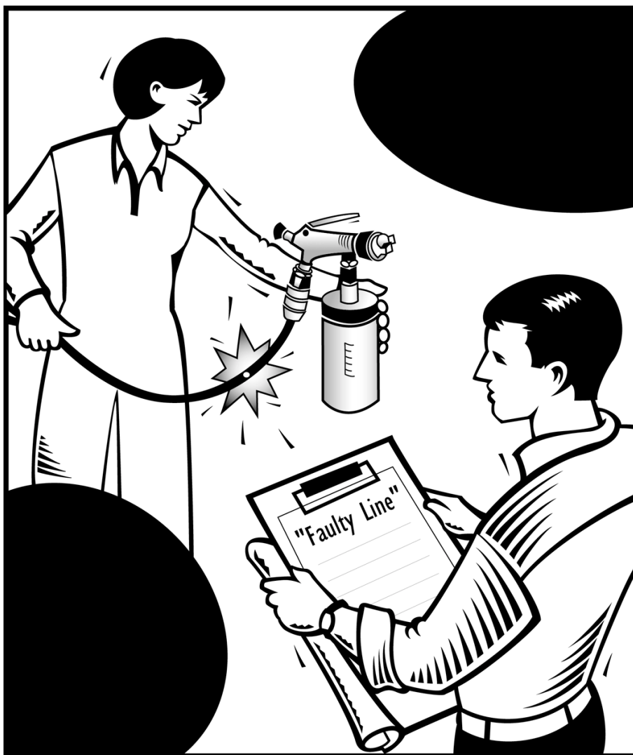
Figure 4 — Inspection of empty spray apparatus shows that there is a hole in the supply line
